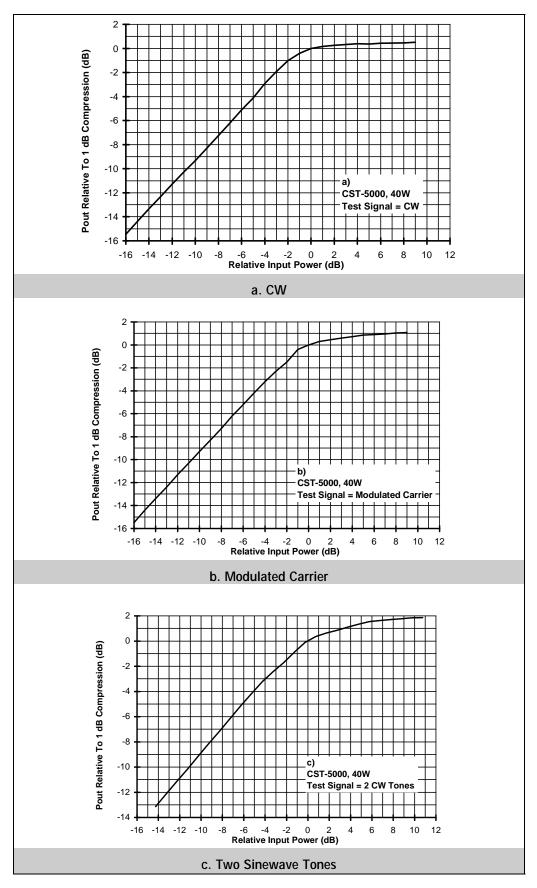
Figure 2. Output Backoff (vs) Input Backoff
