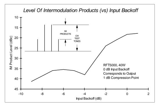
Figure 5. Intermodulation Products (vs) Input Backoff
