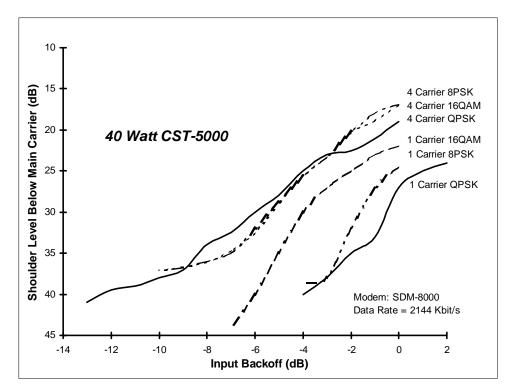
Figure 3. Shoulder Level (vs) Input Backoff
