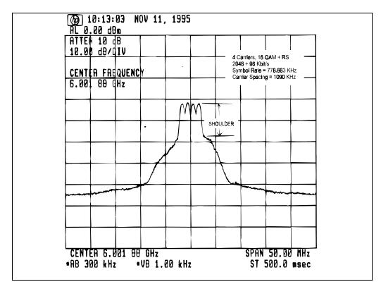
Figure 9. Four Carrier 16QAM
