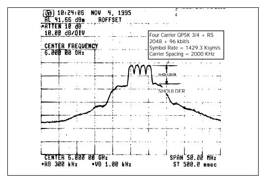
Figure 7. Four Carrier QPSK
