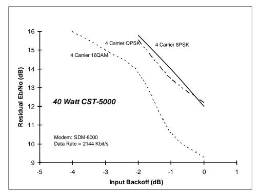
Figure 4. Residual Eb/No (vs) Input Backoff
